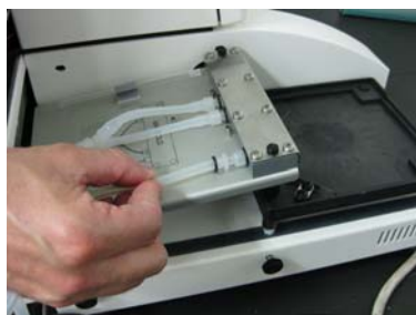
Twist the 2 hose ends ½ turn to the left to facilitate hose attachment
