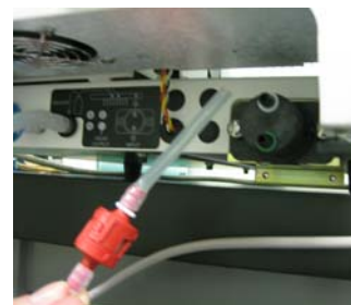
Attachment of media hose to the output of the media pump (top nozzle, white O-rings). Note waste hose connected to vacuum pump connector (left side)
