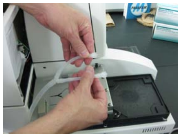
Twist the 2 hose ends ½ turn to the left to facilitate hose attachment
